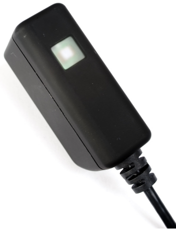
Figure 32: Microswitch light sensor
