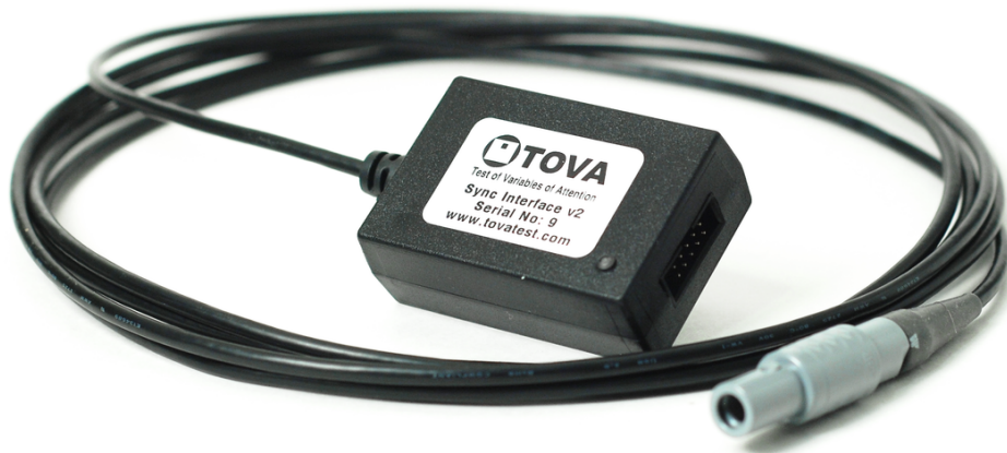
Figure 1: The T.O.V.A. Synchronization Interface
