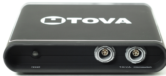
Figure 2: T.O.V.A. USB device with extra front panel connector)
