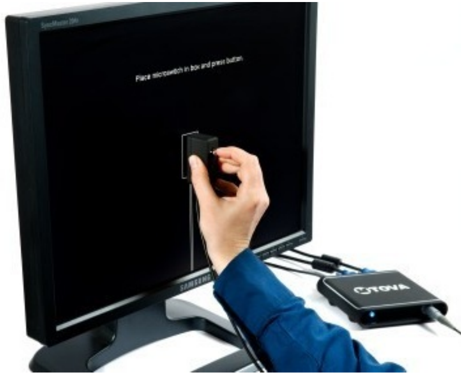
Figure 67: How to hold your microswitch for calibration
