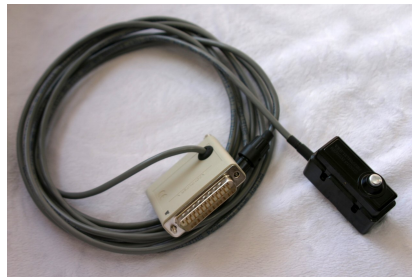
Figure 1: T.O.V.A. hardware for the visual test: the T.O.V.A. microswitch and Scorebox.
