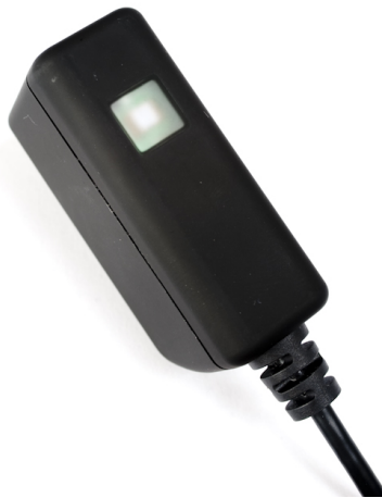
Figure 26: Microswitch light sensor
