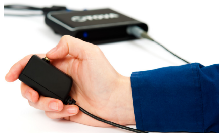
Figure 94: How to hold the microswitch
