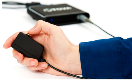
Figure 92: How to hold the microswitch
