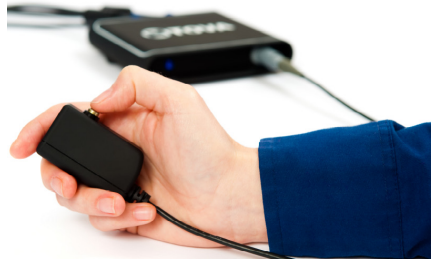
Figure 109: How to hold the microswitch
