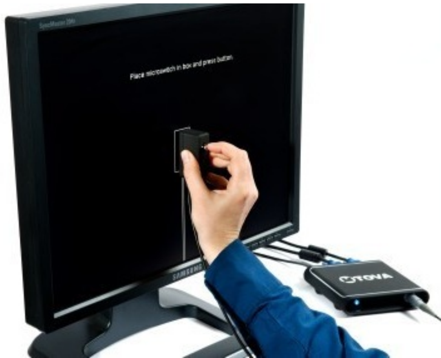
Figure 34: Calibrating the T.O.V.A. to your display.
