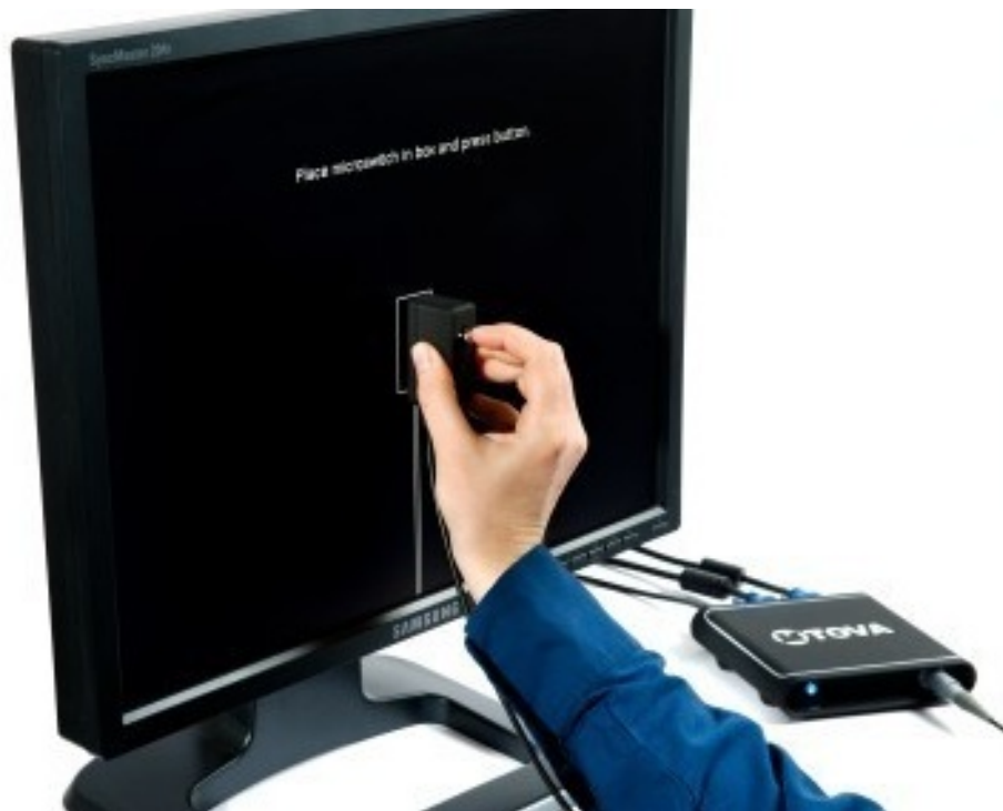
Figure 91: How to hold your microswitch for calibration
